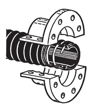
The Bulk-Flex coupling is made of the highest quality cast aluminum. The coupling consists of two halves with internal threads designed to be mechanically attached over the outside of the hose (see illustration below). The Bulk-Flex coupling is designed for a working pressure of 150 PSI. Flange drilling conforms to ANSI 16.5. See page 7 for hose information.
